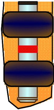
Dual packer type devices have increased flow area compared to a probe.
