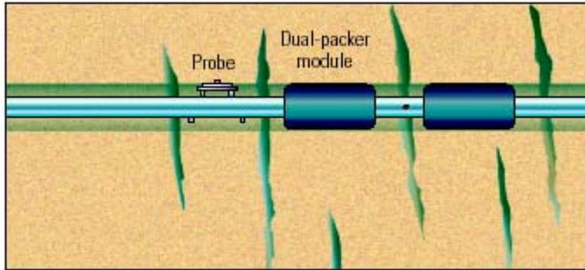
Interval tests conducted show that the fractures are not highly conductive, both packer and probe showing spherical flow
